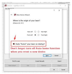
If your decice is support homing, when the homing complete the Laser point is at **Rear Left**, It's not a mistake, because only Rear Left coner can trig homing switch, also the coordinate of device after homing is (maxY, 0), not (0,0), for Master 2 is (170,0).
