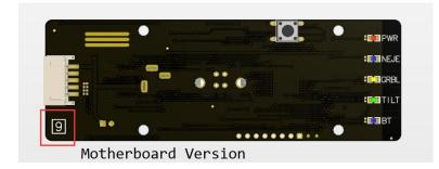
The version of motherboard is 1-10 homing is not support The version of motherboard is 11-12 homing is support
